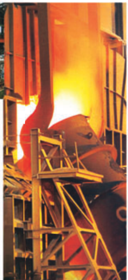
Molten steel being poured into the LD vessel
